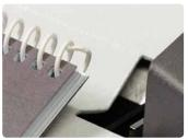
The integrated coil cutting and crimping unit gives the perfect finish to your document every time and crimps the plastic coil at a 45° angle.
